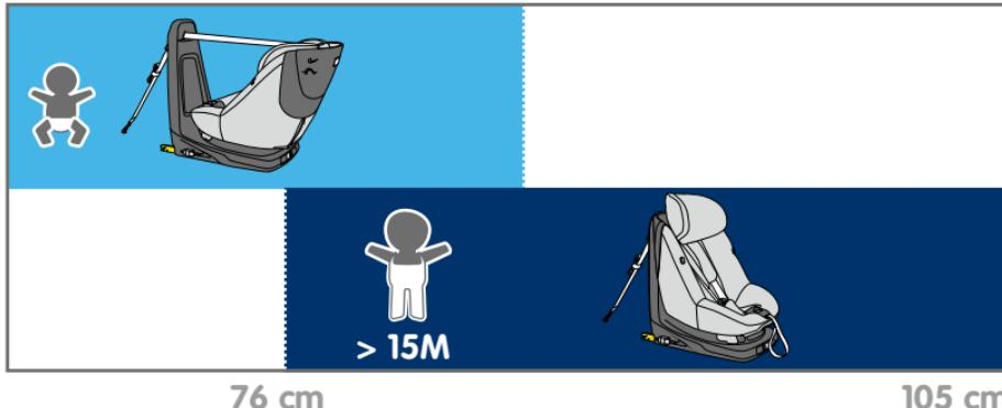
EN - The car seat should be used rearward-facing up to a minimum age of 15 months to guarantee optimum safety for your child. Maxi-Cosi recommends you use the seat in the backward-facing position for as long as possible and up to the limit shown (87 cm). This makes it possible to improve the protection of the head and neck of the infant, which is still very fragile at this age, very significantly.
