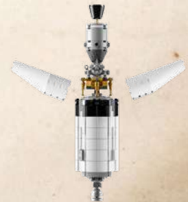
After docking, the CSM pulls the LM away from the launch vehicle's upper stage
