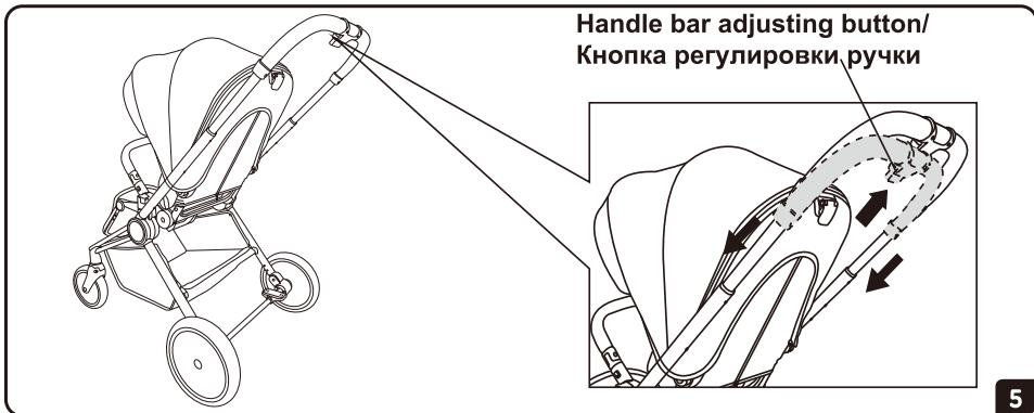
**Hold the button and set the handle in the desired position,
