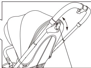
Seat unit adjusting lever/Рычаг
